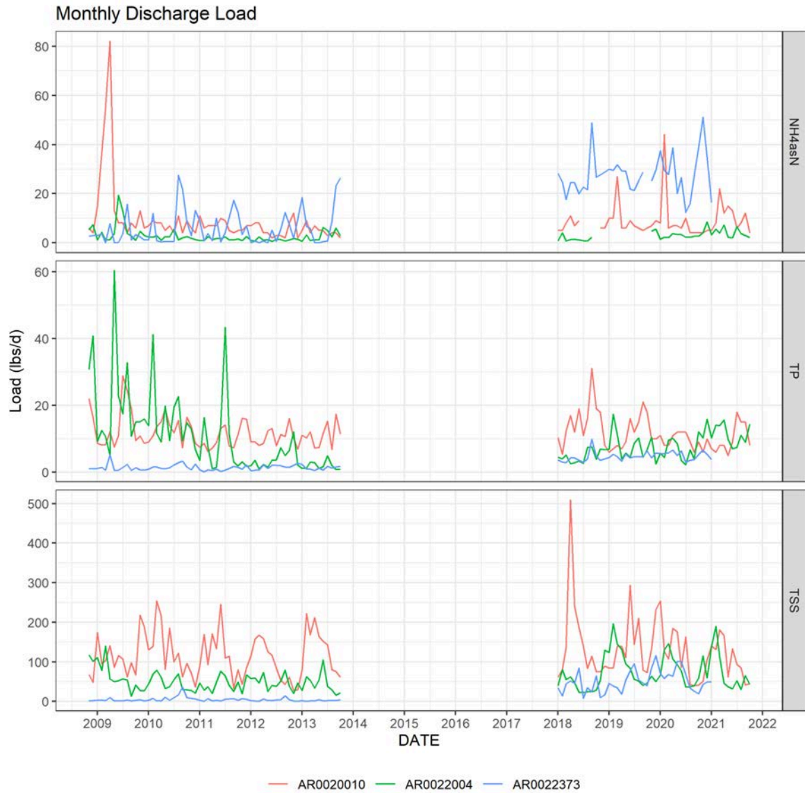
Figure 2-22. Monthly Estimated Pollutant Discharge Loads for the Three Permitted Facilities within Beaver Lake Watershed.
